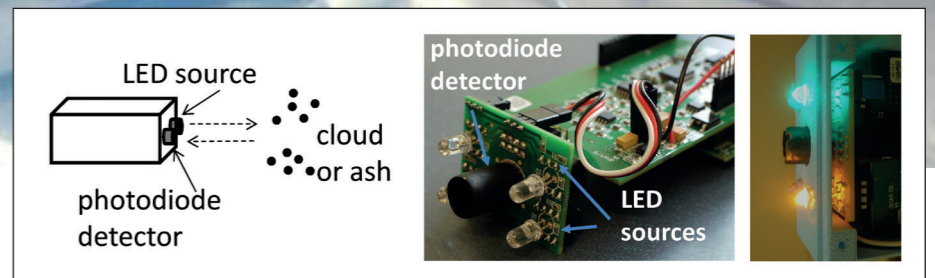
The optical sensor detects droplets and particles in the atmosphere using a high-intensity LED light and a photodiode detector and operates within the VolcLab enclosure
