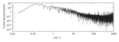
**Figure 15.** A Lomb periodogram of quadratically detrended data collected in the 14.5 h following the annular eclipse on 31 May 2003 (courtesy of Karen Aplin).
