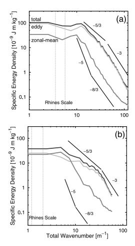
**Figure 4.** Kinetic energy spectra in total wave number  $(2\pi/\text{wavelength})$  for (a) the sloping bottom experiment and (b) the flat bottom case. The Rhines wave numbers for the max/min topographic  $\beta$  are marked by vertical lines. The solid straight lines are references for the slopes, and the -5 line is the theoretical prediction by *Sukoriansky et al.* [2002] with Cz = 0.5.
