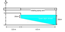
**Figure 1.** Schematic cross-section of the circular container, showing the rotating spray arm used to provide continuous convective forcing. The entire apparatus is set on a circular turntable.
