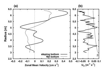
**Figure 3.** Temporally and spatially averaged zonal flow profile (a) and its second derivative with respect to radius (b) for the sloping bottom experiment. The smooth curve in b is the profile of topographic  $\beta$ .
