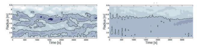
Figure 2: Horizontal velocity field. a, structure and fluctuation of the mean zonal velocity of the mature flow. The contour interval is  $0.2 \text{ cm s}^{-1}$  and the solid line denotes the contour of null velocity. b, initial development of the zonal mean flow in the flat bottom experiment.
