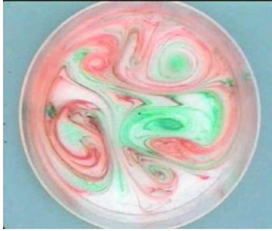
Figure 1.2: Image of two different coloured dyes in a rotating tank of water. As stretching and folding of tracer parcels occurs and filaments form mixing between fluid parcels is inevitable. Image by Prof. J Marshall, Massachusetts Institute of Technology.
