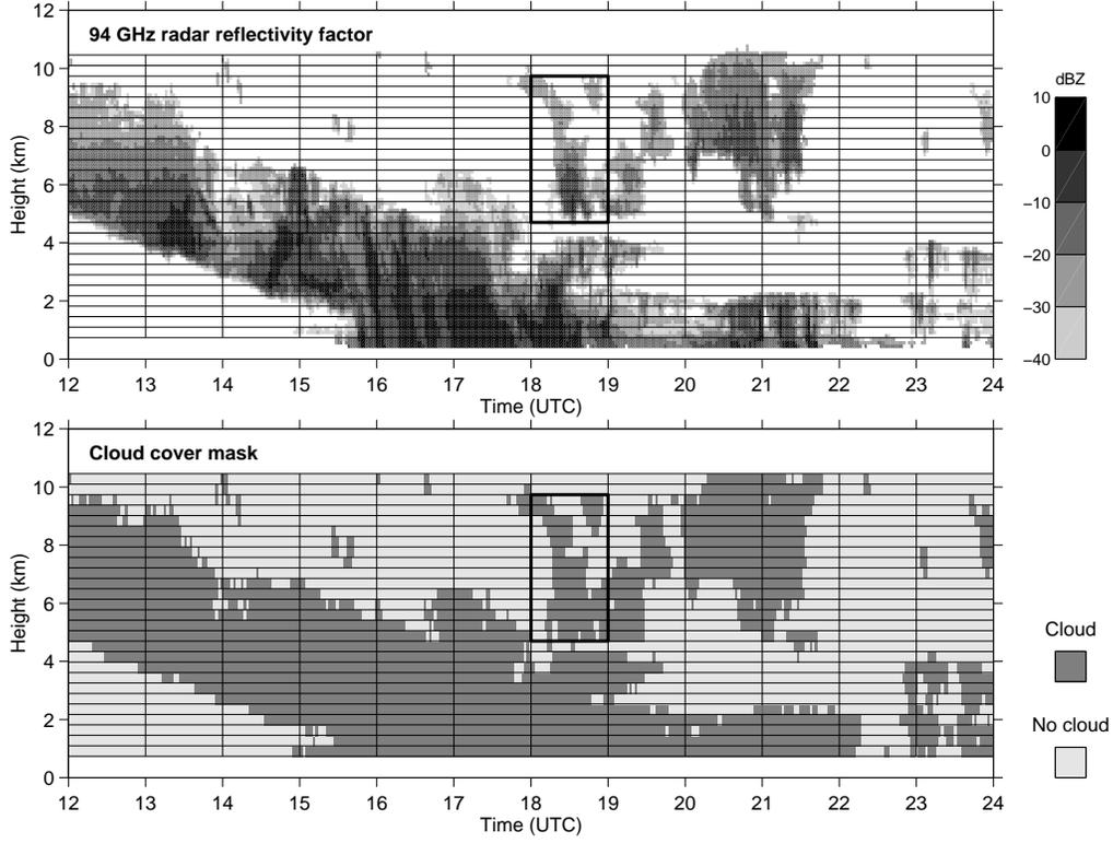
Figure 2. An example of cloud radar data used to derive the cloud cover mask, from 11 December 1998. Intermittent light drizzle was measured at the ground between 17 and 19 UTC. The resolution of the grid is 360 m and 1 hour.
