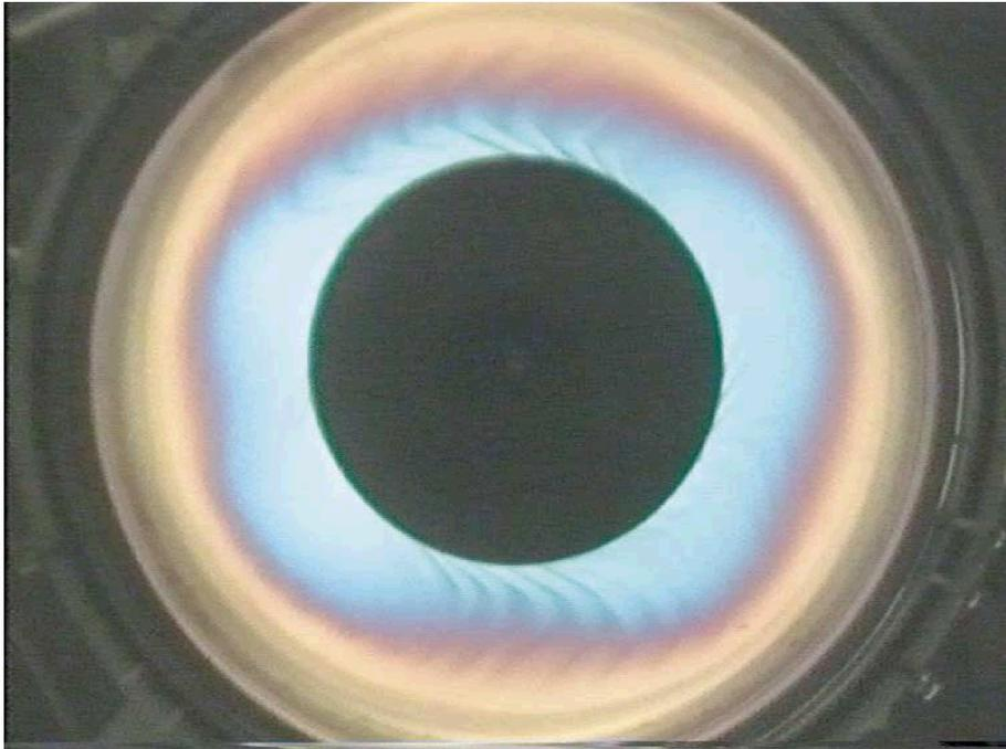
Fig. 3 Experimental image taken by the video camera which views the apparatus in Fig. 1. The tank rotates in the anticlockwise direction. The image can be interpreted by imagining that the North Pole is at the centre, and that the large outer circle represents the equator. A water–oil liquid fills the tank, and different colours in this image correspond to different heights of the interface between the water and oil – blue corresponds to a high interface, and yellow to a low interface.
