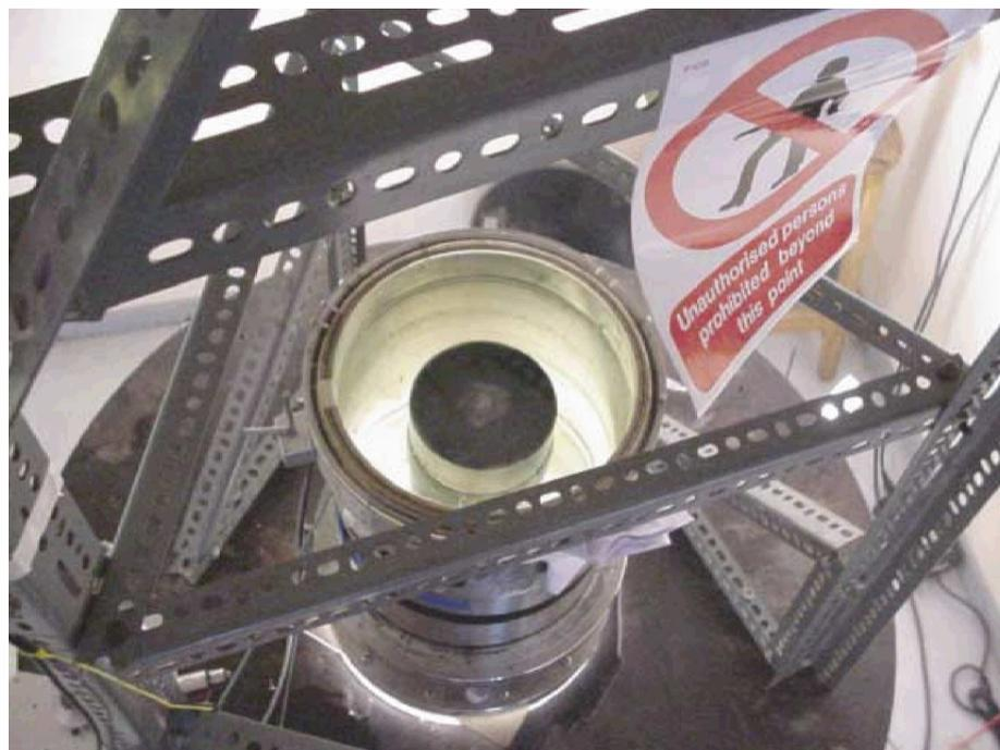
Fig. 1 The laboratory 'teacup', as seen from above. The tank has a transparent glass base and lid. Bright white light illuminates the apparatus from below, and is received by a video camera above. The lid, in contact with the liquid, is made to rotate under computer control relative to the turntable, which also rotates. This provides an instability from which Rossby-type waves can grow.
