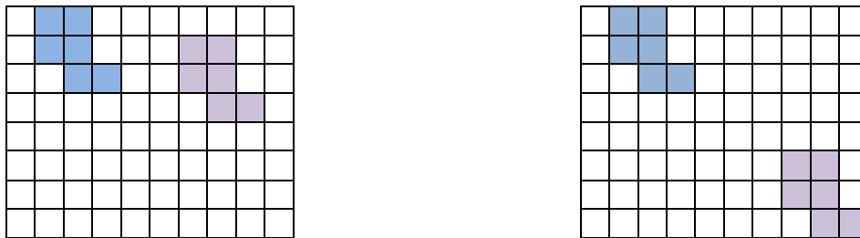
Figure 1: The double penalty problem, means that errors in the location of a band of precipitation are counted twice, once where the model shows the precipitation and once where the observations locate the precipitation. The observations are shown in blue and the forecast in purple. Therefore, both forecasts shown in this figure are considered equally incorrect and the best results would come from not providing a forecast at all.
