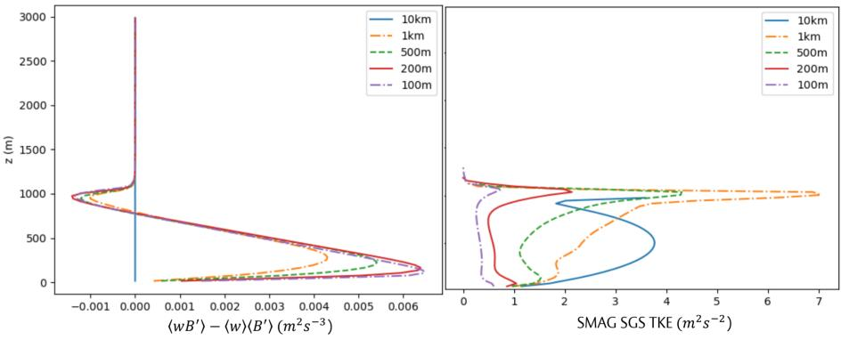
**Figure 3**. Horizontal profile of hourly mean, horizontal averaged buoyancy production rate of KE (left) and Smagorinsky sub-grid scale TKE (right) after 1h of spinning up.
