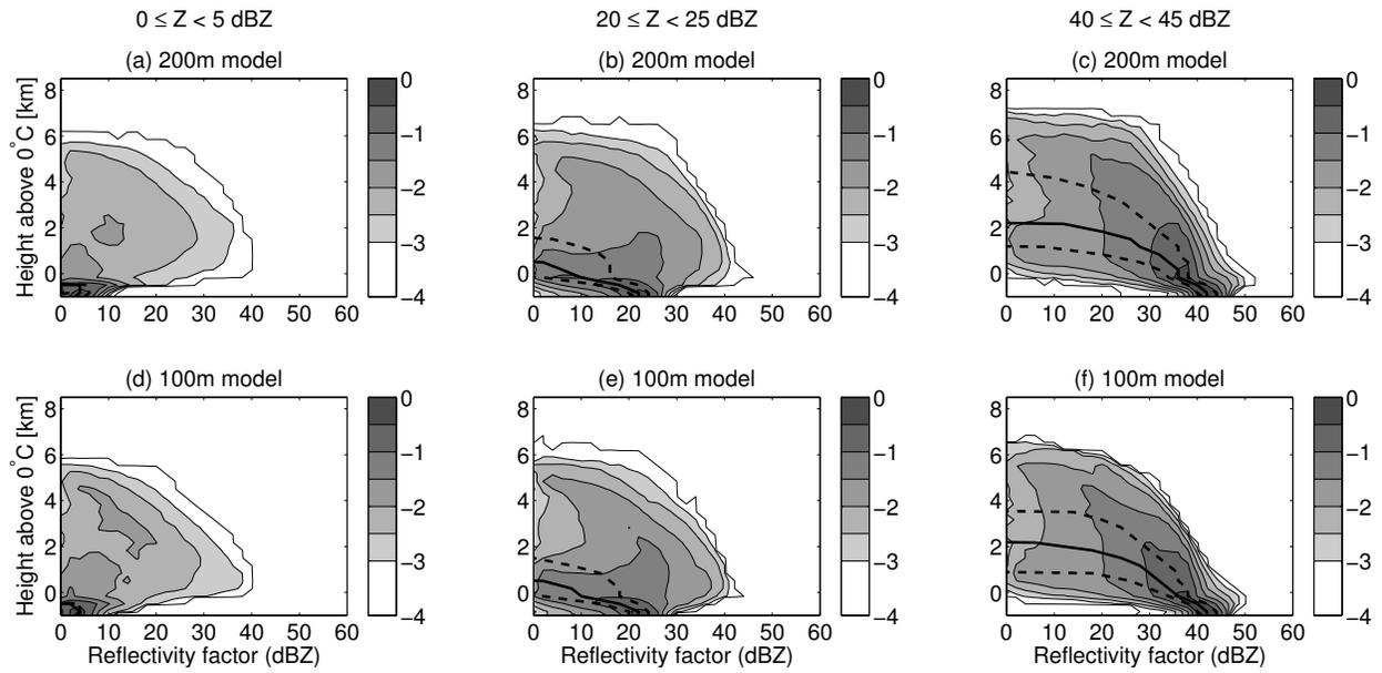
FIG. 8. As in Figure 7, but for UM at 200-m grid length (first row), UM at 100-m grid length (second). Both simulations were run with 140 vertical levels. The 100-m simulation was analysed on a smaller domain of  $140 \times 140$  km.
