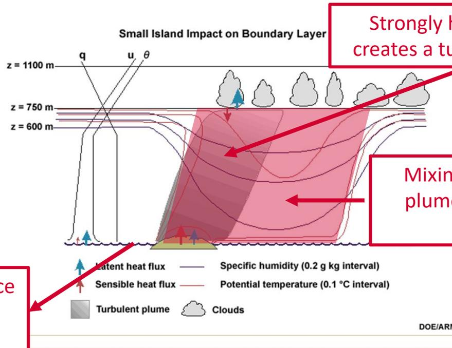
Strongly heated island creates a turbulent plume
