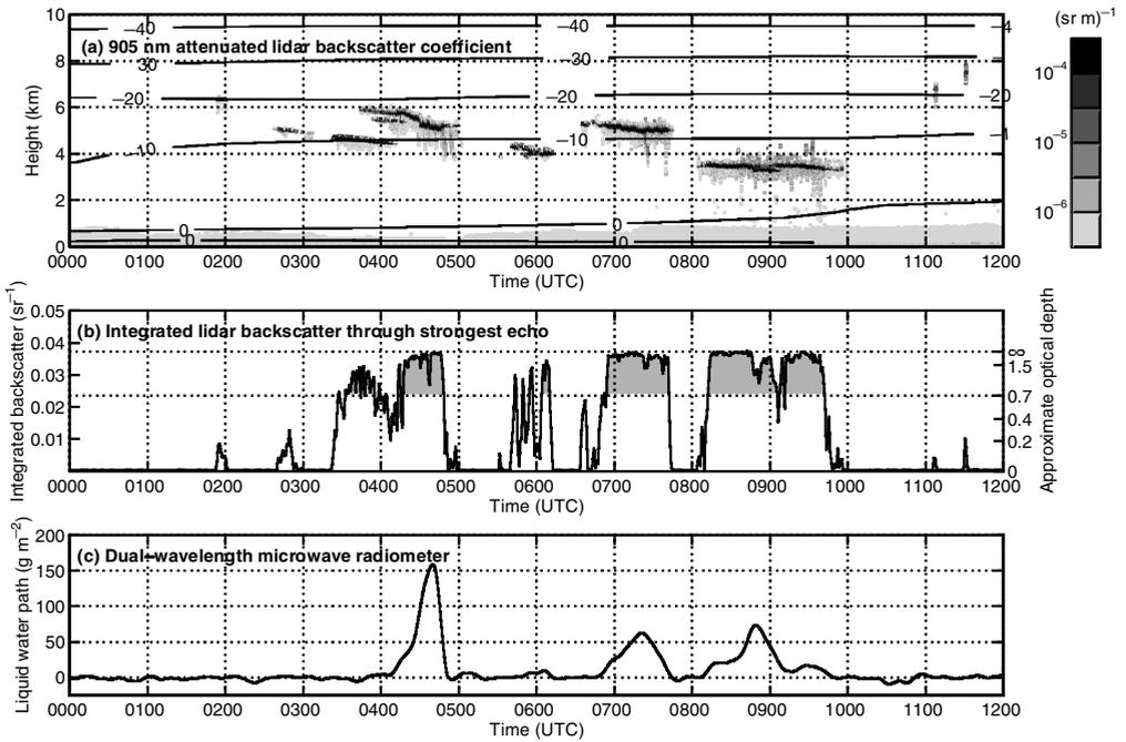
Figure 2. Supercooled-water detection on 10 November 2001: (a) attenuated backscatter coefficient, (b) the approximate optical depth of the layer, as in Fig. 1, and (c) liquid-water path retrieved using a dual-wavelength microwave radiometer.
