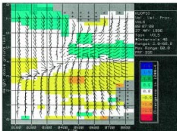
FIG. 3. Time–height cross section of VVP wind soundings derived from the Finnish Doppler radar at Kuopio at 0100–0800 UTC 27 May 1996. The color background exhibits the radar derived distribution of divergence  $10^{-4} \text{ s}^{-1}$ . Crosses indicate points where the signal is either too weak or does not pass the quality thresholds as, for example, signal coherency. The case is related to a passage of deepening frontal wave followed by cold air advection.
