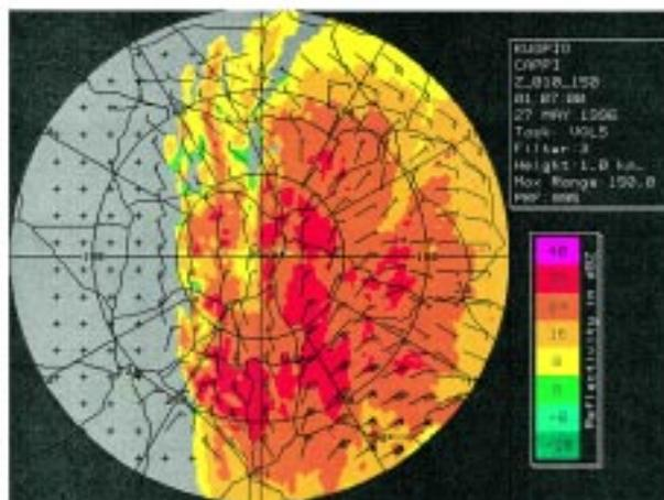
FIG. 4. Horizontal wind field at the constant altitude plan position indicator (CAPPI) height of 1 km, derived by VVP processing in 30 km long and  $30^\circ$  wide volume segments, and then interpolated to a grid of  $10 \text{ km} \times 10 \text{ km}$  resolution at the Kuopio Doppler radar at 0107 UTC 27 May 1996. The color background exhibits the slightly smoothed dBZ field at the CAPPI height of 1 km.
