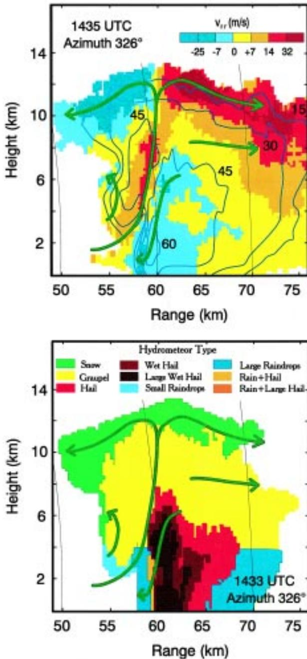
FIG. 6. Vertical section (RHI) taken by POLDIRAD through the center of a severe hailstorm that occurred in southern Germany on 30 June 1990 (see Höller et al. 1994). The upper panel shows storm-relative radial velocity  $v_r$  overlaid by reflectivity contours (solid lines) labeled in dBZ. The lower panel indicates the different types of hydrometeors as derived from  $Z_{DR}$  and LDR measurements taken 2 min earlier at the same azimuth. The bold arrows illustrate possible streamlines.
