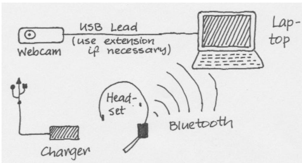
Figure 2: Setup of the Blue kit. In case a DSL camera is used, the headset should be used as shown. In case the computer does not have Bluetooth, the headset can be connected to a Bluetooth dongle which is plugged into a USB port (this still needs to be procured).
