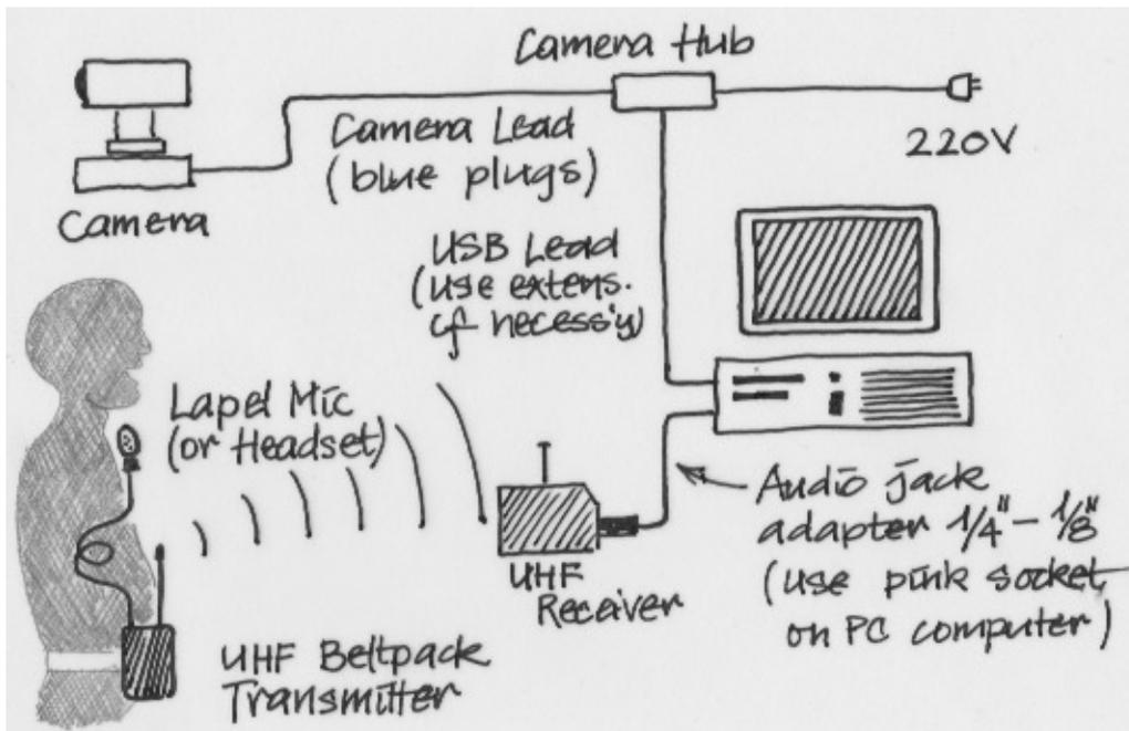
Figure 1: Setup of the yellow kit. In case a DSL camera is used, the microphone can be used as shown, or alternatively the audio jack can be plugged into the camera, provided it has an 1/8" analog audio input.
