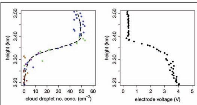
Above: Left – cloud droplet number concentration at the base of the cloud. Right – voltage on the charge sensor electrode as it descended through the cloud. The change in electrode voltage at cloud base indicates the presence of charge in this region. Theory predicts that stratiform clouds should be charged at their upper and lower edges
