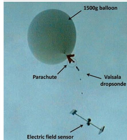
Above: Balloon developed at Reading, and flown successfully using this data acquisition and retrieval system
