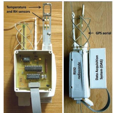
Above: The Data Acquisition System (DAS) developed at the University of Reading to interface additional sensors to the Vaisala RS92 radiosonde. The DAS allows data from additional sensors to be sent across the radio link synchronous with the standard meteorological parameters measured by the RS92 (P,T,U and GPS).
