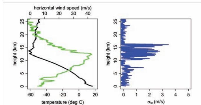
Above: Left - vertical profiles of temperature (black) and horizontal wind speed (green) measured by the standard sensors on a Vaisala RS92 radiosonde. Right – vertical profile of variability in vertical wind speed measured on the same flight by the Reading turbulence sensor data – note the more detailed structure in the turbulence sensor data than from the horizontal wind speed inferred from GPS measurements made by the RS92
