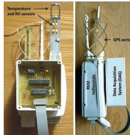
Above: The Data Acquisition System (DAS) developed at the University of Reading to interface additional sensors to the Vaisala RS92 radiosonde. The DAS allows data from additional sensors to be sent across the radio link synchronous with the standard meteorological parameters measured by the RS92 (P,T,U and GPS).
