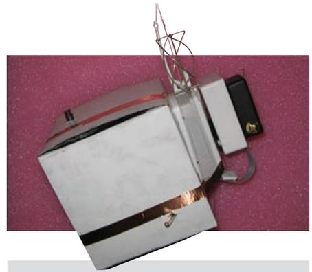
Above: An RS92 radiosonde instrumented with a charge sensor (right) and aerosol particle counter (left). The specially developed data acquisition system allows the extra sensor data to be transmitted back to the surface over the radio link, synchronously with the standard meteorological data measured
