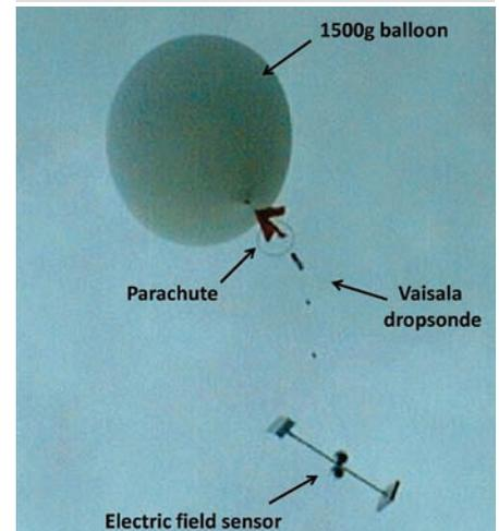
Above: Balloon developed at Reading, and flown successfully using this data acquisition and retrieval system
