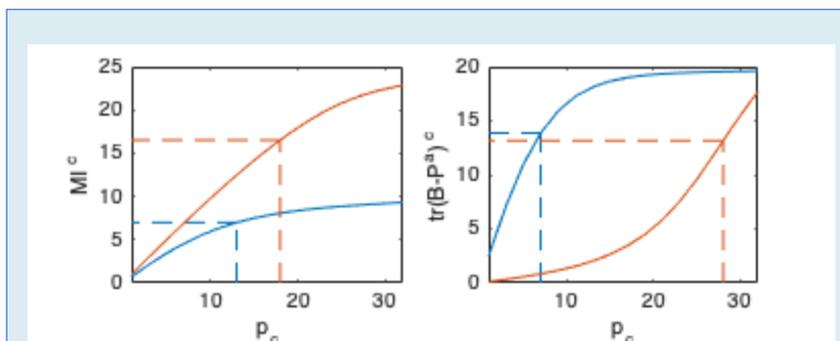
Fig 1.  $MI^c$  (left) and  $\text{tr}(\mathbf{B} - \mathbf{P}^a)^c$  (right) vs number of compressed observations assimilated ( $p_c$ ).  $\mathbf{B}$  and  $\mathbf{R}$  are given by circulant matrices with SOAR correlation functions. The length scales in  $\mathbf{B}$  are 5 and the length scales in  $\mathbf{R}$  are 0.1 (blue) or 10 (red). Adapted from Fowler 2019.
