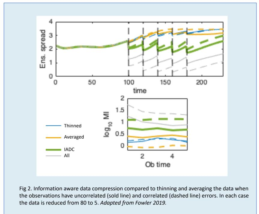
Fig 2. Information aware data compression compared to thinning and averaging the data when the observations have uncorrelated (solid line) and correlated (dashed line) errors. In each case the data is reduced from 80 to 5. Adapted from Fowler 2019.
