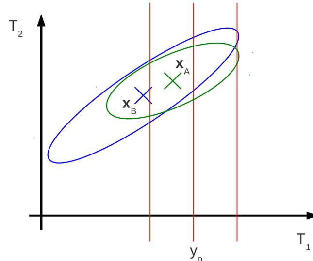
$$\underbrace{P(\mathbf{x} = \mathbf{x}_t | \mathbf{y}_o)}_{\text{posterior}} \propto \underbrace{P(\mathbf{y}_o | \mathbf{x} = \mathbf{x}_t)}_{\text{likelihood}} \times \underbrace{P(\mathbf{x} = \mathbf{x}_t)}_{\text{prior}},$$
