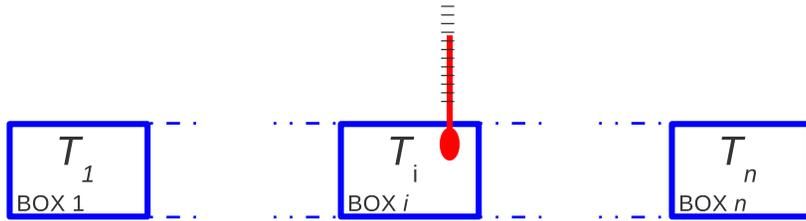
$$\mathbf{x} = \begin{pmatrix} T_1 \\ \vdots \\ T_i \\ \vdots \\ T_n \end{pmatrix}, \quad \mathbf{x}_B = \begin{pmatrix} T_{B1} \\ \vdots \\ T_{Bi} \\ \vdots \\ T_{Bn} \end{pmatrix}, \quad \mathbf{y}_o = (y), \quad \mathcal{H}(\mathbf{x}) = T_i,$$
