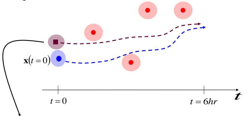
Since the model is perfect, the **initial condition determines the whole trajectory**.
