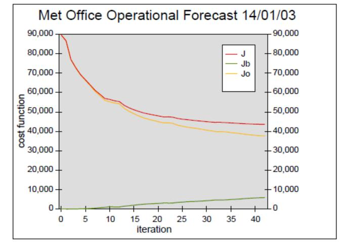
Value of the cost function and its components as a function of **iteration** for Met Office © 3DVar.
