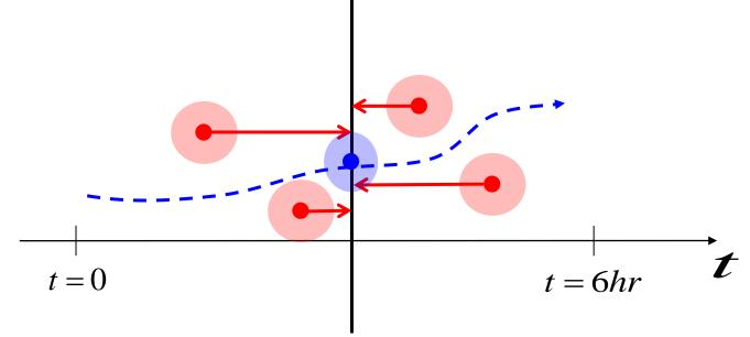
b) Find a trajectory that fits the observations throughout the whole forecast window. This is 4DVar: we have added an extra dimension to the minimization. Two flavours: strong constraint and weak constraint.
