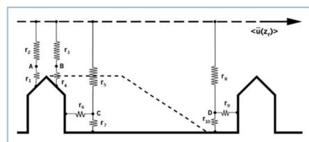
Figure 4. The new resistance network for a steeply pitched roof. For the street surface, only the resistances 5, 7, 8 and 10 are active.
