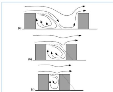
Figure 1. Flow patterns around street canyons for different aspect ratios (building height to street width,  $H/W$ ) (Harman et al., 2004; Oke, 1987). From a) to c), the flow regimes represented are the isolated roughness regime, the wake interference and the skimming flow regime, respectively.
