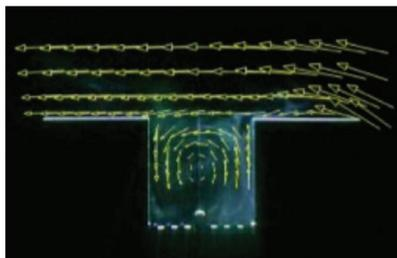
Figure 3a. Flow visualisation for a street canyon with flat roofs. Mean velocity field indicated by the arrows.
