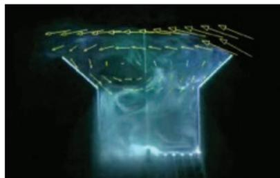
Figure 3b. Flow visualisation for a 45° pitched roof. The roof level vortex can be clearly seen. The indication of poorer ventilation can be noted by the higher concentration of tracer gas near the surface. (Thanks to B. Leitl at University of Hamburg for use of wind tunnel facilities).
