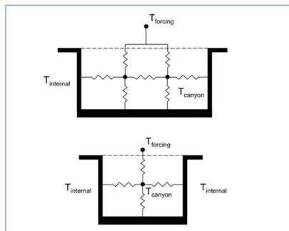
Figure 2. The Arup OutdoorRoom (ODR) resistance network model for heat transfer in a street canyon. Internal, canyon and forcing temperatures are indicated.
