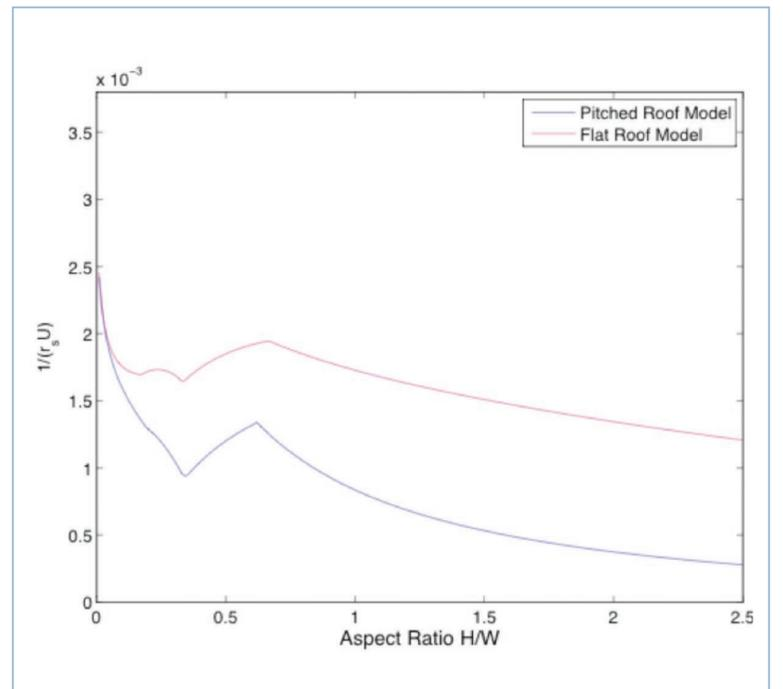
Figure 5. The influence of changed roof pitch on the resistance to heat transfer. The magenta line depicts the inverse of the resistance (non-dimensionalised by wind-speed  $U$ ) for transfer from the street surface with a flat roof (Harman et al., 2004) and the blue line represents the results with the new pitched roof parameterisation.
