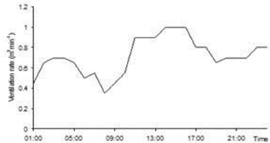
Figure 4 – Infiltration rates for room 1 on 28 th Nov 2011 calculated from NO x data using inverse MIAQ method.
