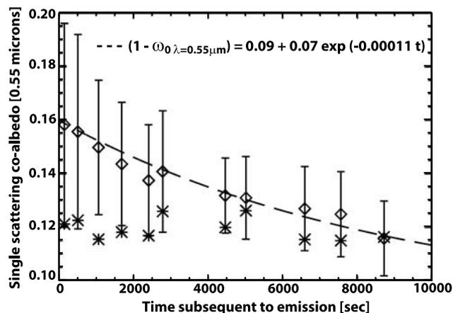
**Figure 2.** Evolution of the aerosol co-albedo downwind of the fire. Diamonds represent the mean value for each cross plume transit measured with the PSAP and nephelometer. Error bars are the standard deviation from this mean. Values using the PCASP size distribution for each transit and Mie calculations ( $n = 1.54 - 0.018i$ ) are shown with an asterisk. The exponential fit suggests that it will take 5 hours for the co-albedo to reach 0.10, which is representative of the aged regional haze.
