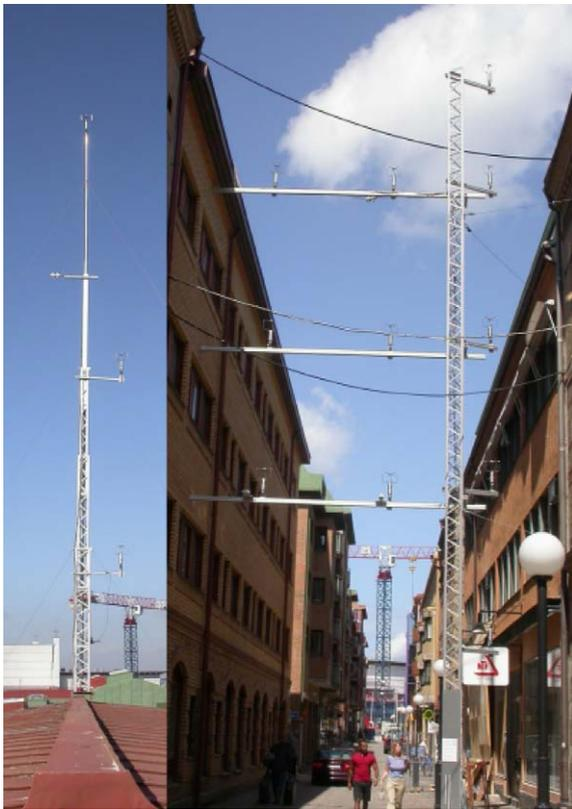
Fig. 3. Photos of the masts and instrumentation: roof level (left) and canyon (right).
