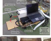
KCL's FTIR emissivity kit (*left*) can measure the thermal radiance of surfaces (*below*). By calibrating the spectrometer using target surfaces of known radiance (blackbodies) and eliminating background radiation (using a gold plate), emissivity spectra (*right*) can be computed.
