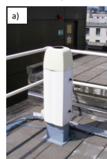
Figure 2: a) Vaisala CL31 Ceilometer located at KSS. b) Ceilometer density plot from a cloudless day (Dec 7th 2008). Notice the clear distinctive layer near the surface which indicates high air pollution concentrations the top of which is the MLH.
