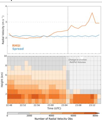
Time series of (top) posterior radial velocity RMSI and ensemble spread ( $m s^{-1}$ ) and (bottom) number of observations per 500 m vertical bin for each assimilation cycle.
