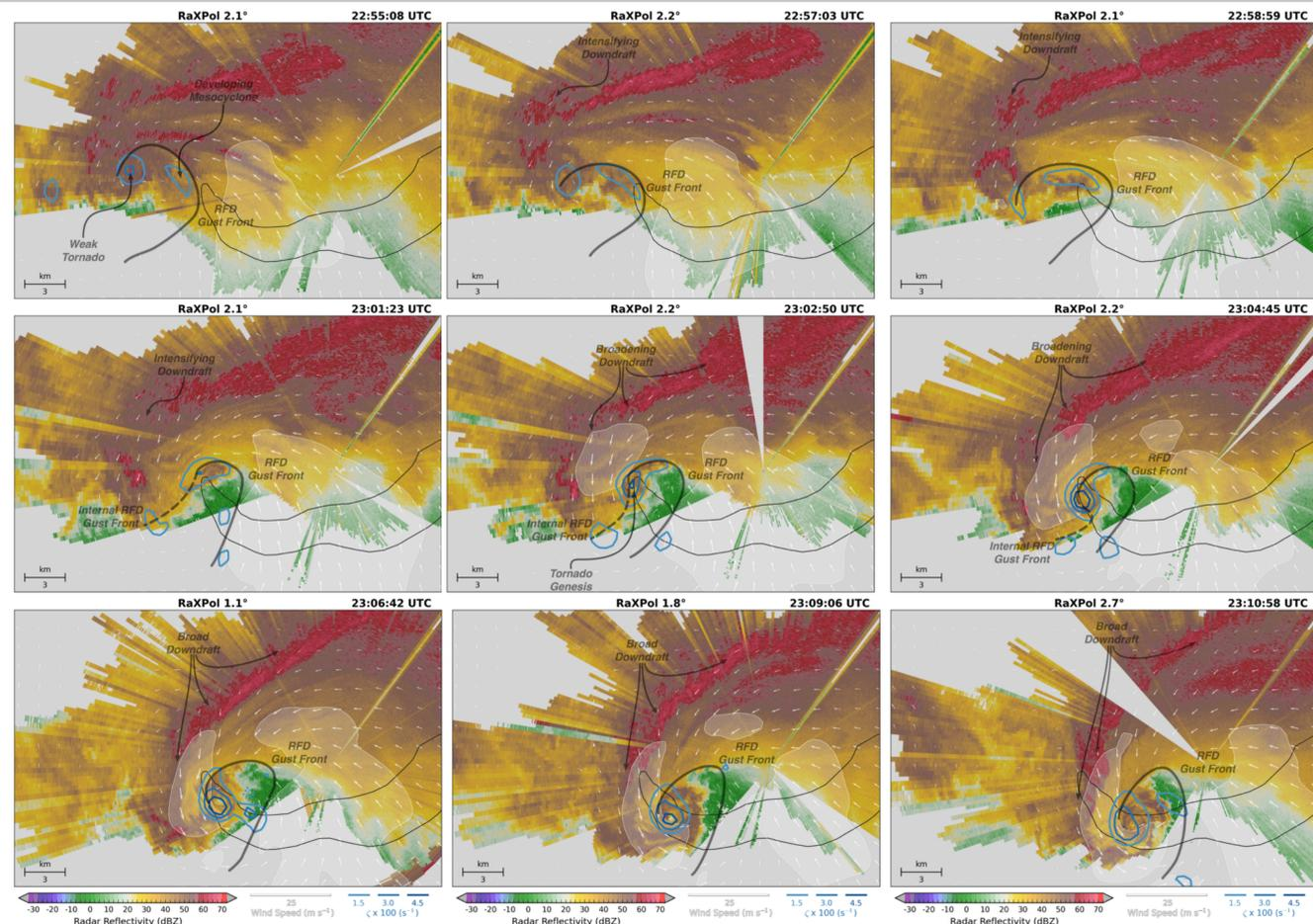
RaXPol reflectivity with ensemble mean vertical vorticity ( $s^{-1}$ ) at 437 m AGL and wind vectors at the lowest model level overlain. Wind speeds greater than  $25 m s^{-1}$  are shaded white, thin black lines denote the damage track of the El Reno tornado, and prominent storm features are annotated.
