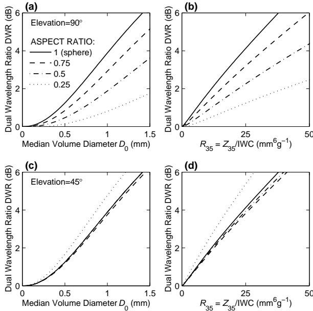
FIG. 2: DWR as a function of  $D_0$  and  $R_{35}$  at vertical incidence (top row) and at an elevation of  $45^\circ$  (bottom row), for oblate crystals of four different aspect ratios. The radiation is vertically polarized at both wavelengths and the distribution is exponential.
