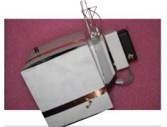
Above: An RS92 radiosonde instrumented with a charge sensor (right) and aerosol particle counter (left). The specially developed data acquisition system allows the extra sensor data to be transmitted back to the surface over the radio link, synchronously with the standard meteorological data measured
