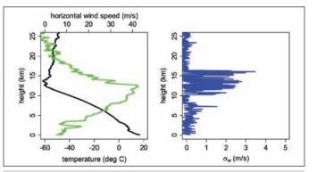
Above: Left - vertical profiles of temperature (black) and horizontal wind speed (green) measured by the standard sensors on a Vaisala RS92 radiosonde. Right – vertical profile of variability in vertical wind speed measured on the same flight by the Reading turbulence sensor – note the more detailed structure in the turbulence sensor data than from the horizontal wind speed inferred from GPS measurements made by the RS92
