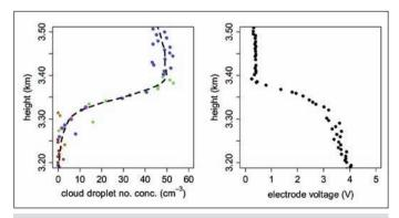
Above: Left – cloud droplet number concentration at the base of the cloud. Right – voltage on the charge sensor electrode as it descended through the cloud. The change in electrode voltage at cloud base indicates the presence of charge in this region. Theory predicts that stratiform clouds should be charged at their upper and lower edges
