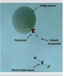
Above: Balloon developed at Reading, and flown successfully using this data acquisition and retrieval system
